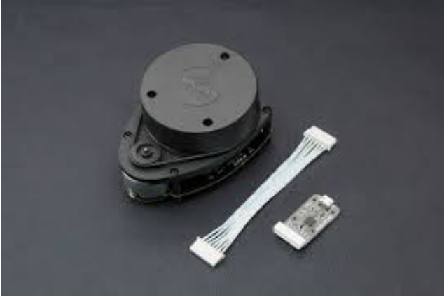
Figure 1.2: RPLidar A1M8 with connectors to integrate with Linux systems
