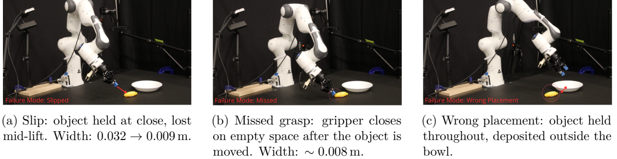
Figure 2: Representative frames of the three deliberately induced failure modes. Red markers indicate the location of the banana at the moment of failure; green markers indicate the intended target.
