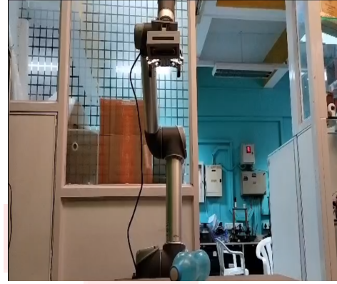
(b) UR5 Hardware Setup for Graspnet
